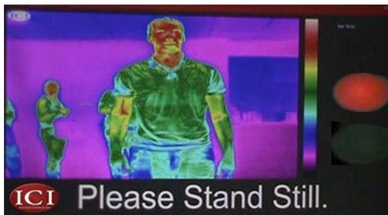
IR Fever Scanner display. Passengers are told to remove hat and glasses and to stand still. A red light and audible alarm signals screener that a passenger's skin temperature is elevated above a set level. That person is pulled aside for further screening to see if there actually is a fever present.
